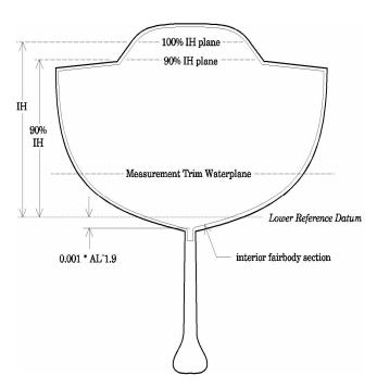
All types of cut-outs and fitting recesses penetrating into the volume defined by 3 and 4 are forbidden. Only control lines may pass into the coach-roof volume.
