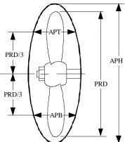
**APT** and **APB** are the maximum aperture widths measured parallel to the propeller shaft, found not less than PRD/3 above and below the shaft centerline.
