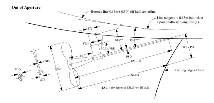
\*ST3 is the maximum strut width measured parallel to the propeller shaft found not more than 0.3 x PRD above the shaft centerline.
