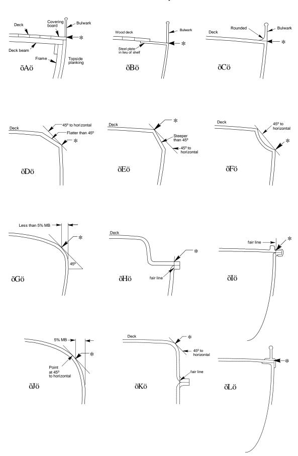
B2.4 If the sheer points on the freeboard stations can not be taken, they may be selected on different points in which case vertical distances shall be recorded in the hull offset file as:
